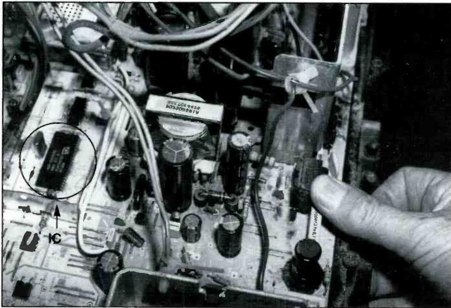
**Figure 6.** The sound circuits in several RCA TV chassis might be included with the chroma, luma, and deflection circuits in a single large IC processor.
