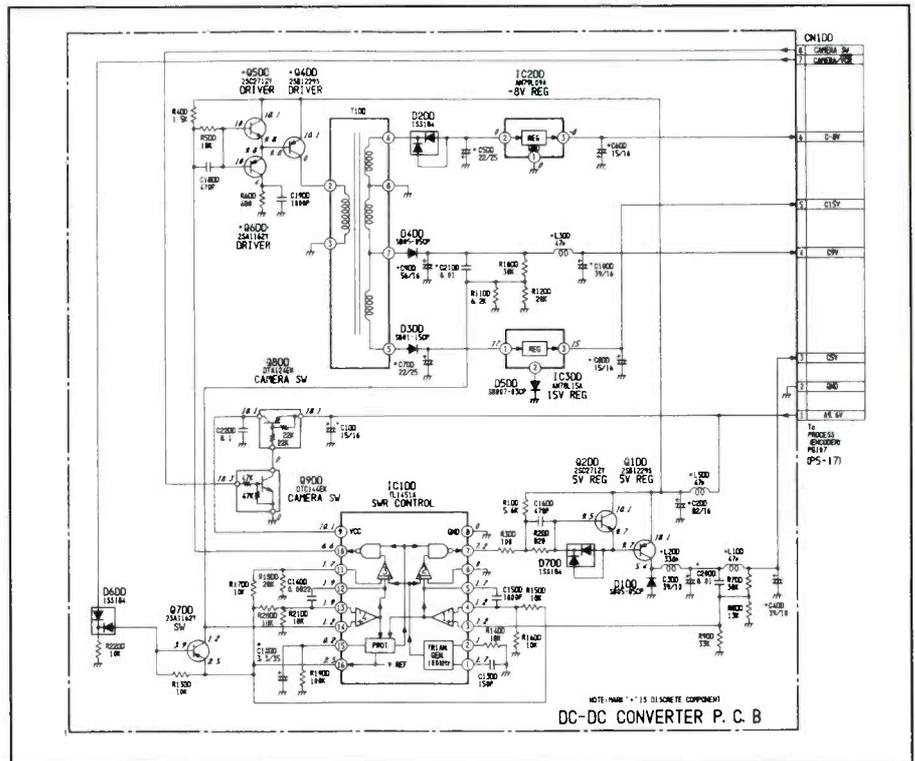
Figure 1. A camcorder, which is portable, is different from a VCR in that it needs a dc-to-dc converter to convert the battery voltage into the various voltages required by the circuitry.
