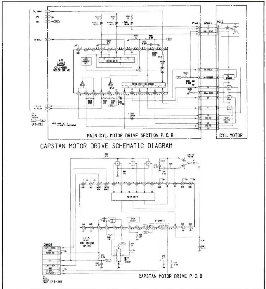
**Figure 9.** Called a mode motor in some camcorder designs, the capstan motor establishes the tape movement in the play, record, rewind, fast forward, and search modes. Typically, the motor will drive mechanical assemblies through either gear or belt-driven mechanisms. The circuits that provide the drive signals for the capstan motor are found in this circuit, and the capstan motor drive section of the main circuit board.
