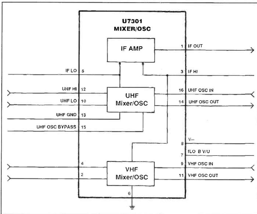
**Figure 3.** If you encounter a CTC187 for which the tuner is inoperative on all cable channels, try tuning UHF channels. If you get good picture and sound, you know that at least a part of the tuner is working and that the problem will be in the oscillator-mixer, or the tuner controller, or related circuitry.
