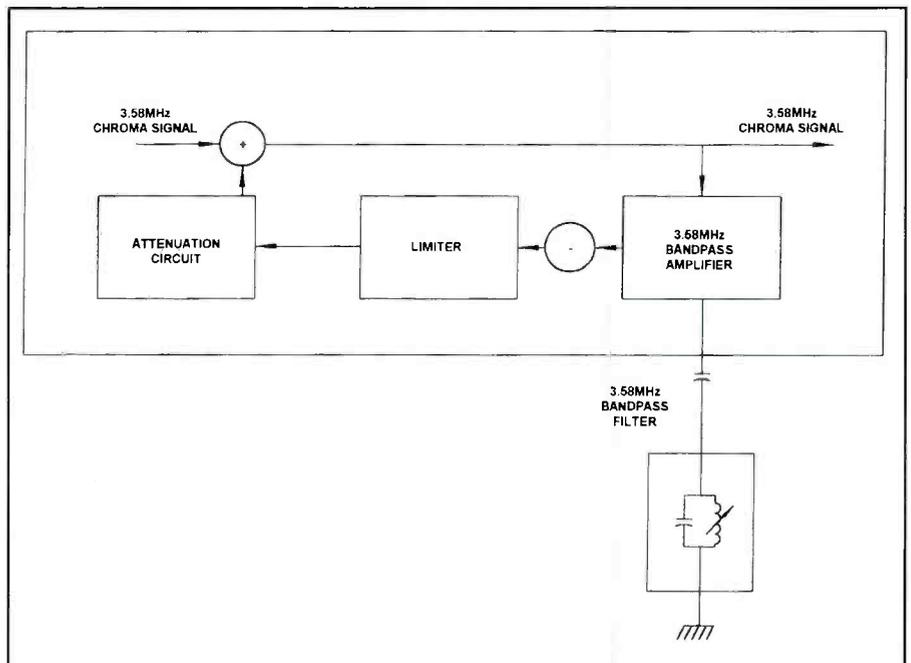
**Figure 5.** The chroma deemphasis circuit in a camcorder provides an equal and opposite effect on the chroma signal as that caused by the preemphasis circuit.
