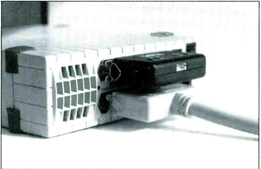
**Figure 3.** When you encounter a problem on a SCSI bus, always first inspect, and then test the cables, since they are the easiest part of the Bus to test. Check the cables for cracks and breaks, especially around the strain relief.
