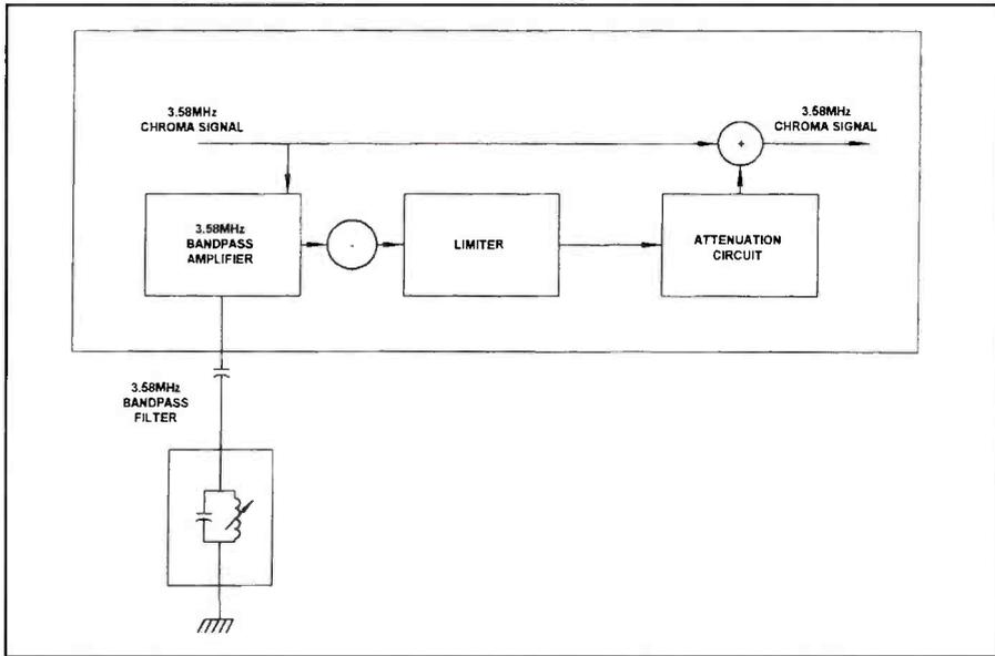
**Figure 4.** Chroma circuits in camcorders contain preemphasis circuits that give little emphasis to frequency components close to the 3.58MHz center frequency and higher amounts of emphasis to frequency components at the upper and lower ends of the band. As shown here, the 3.58MHz signal feeds directly toward the summing point while also branching to the 3.58MHz bandpass amplifier. The output signal from the bandpass amplifier is the 3.58MHz center frequency.
