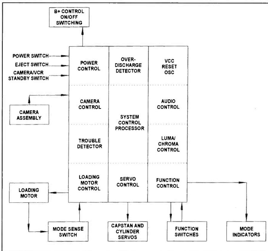
**Figure 7.** As shown in this block diagram, different parts of the control processor maintain the functions of the VCR and camera assemblies. With the VCR portion of the control system, the loading motor control area drives the motor and circuitry that engages levers and gears that control the mechanical operation of the video cassette recorder.
