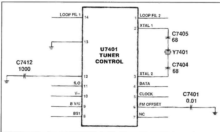
**Figure 2.** Crystal Y7401 develops the reference signal for the tuner controller IC, IC7401. Look for a 4MHz signal at about 1V<sub>PP</sub>. A defective crystal will cause one of two problems: a completely dead tuner or one that drifts off frequency.
