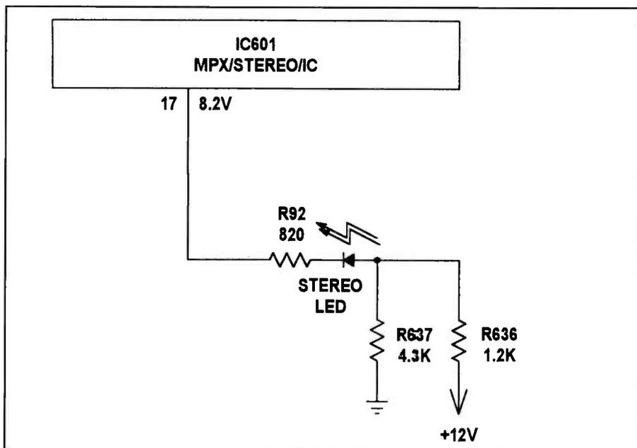
**Figure 10.** Replace IC601, the stereo/multiplex integrated circuit, in a Goldstar CMT-2612 when the sound and the LED stereo light cut in and out.
