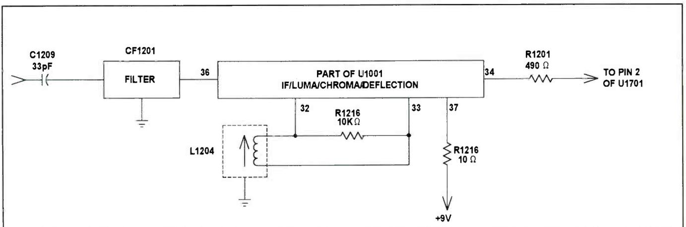
Figure 5. CF1201, L1204, and U1001 can all be causes of hum and buzzing noises in the RCA CTC166, and CTC167 chassis.
