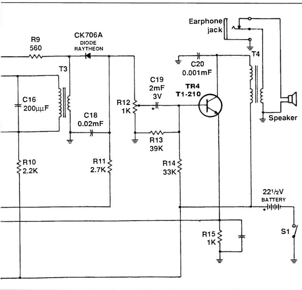
← **Figure 2.** Schematic diagram of Regency Model TR-1. The TR-1 is a superheterodyne circuit using germanium transistors supplied by Texas Instruments. The diode detector was a germanium diode supplied by Raytheon (CK 706A) and in some radios Tungsol (TS 117) were used.
