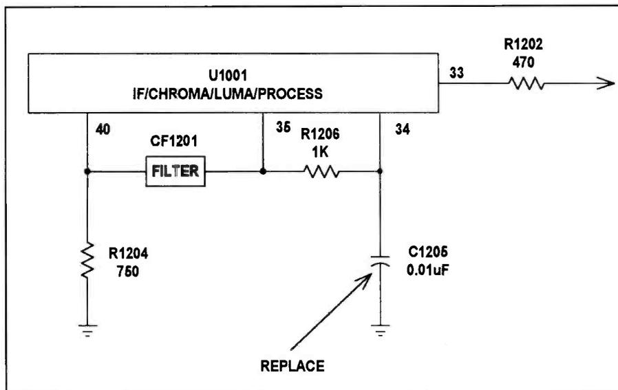
Figure 8. In the RCA CTC159 chassis, C1205 may be the cause of the symptom of no sound.
