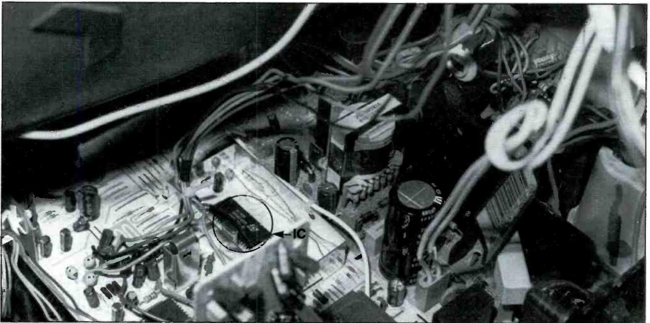
Figure 2. The stereo microcontroller, multiplex decoder, and multiplex demodulator in one of these sets might be included in a single large IC.
