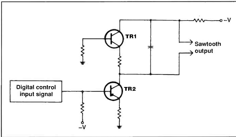
Figure 3. G.B. Herzog's frequency-controlled oscillator.
