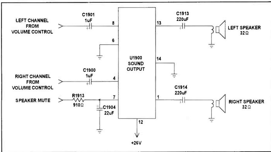
Figure 4. The dual sound output IC (U1900) can cause many different audio problems.
