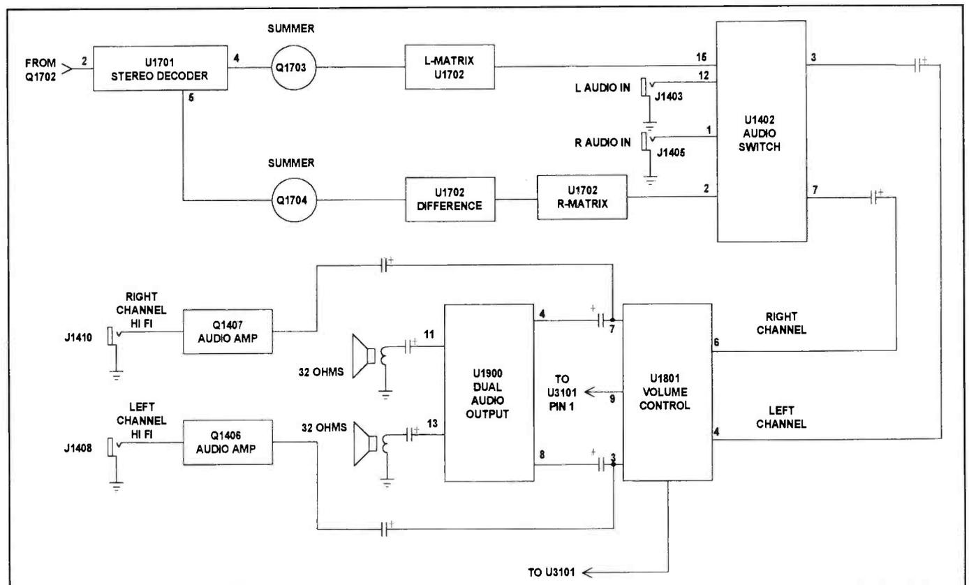
Figure 1. A block diagram of the stereo circuits in the RCA CTC166 television chassis.
