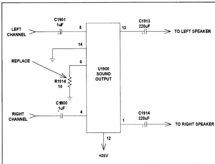
Figure 9. After replacing integrated circuit U1900 to cure extreme audio distortion, check R1914 to see if it is open or burned or otherwise damaged.
